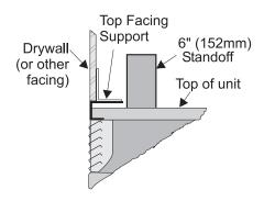
Install Side Nailing Strips, Top Facing Support, and Top Standoffs before unit is slipped into position. See page 9 for assembly details.
